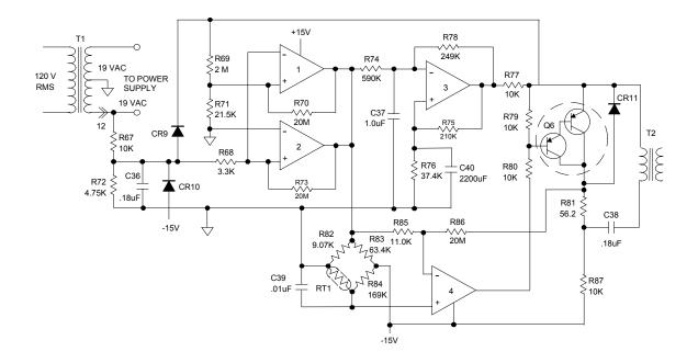
Figure 5-3. Case Heater Control Circuit
